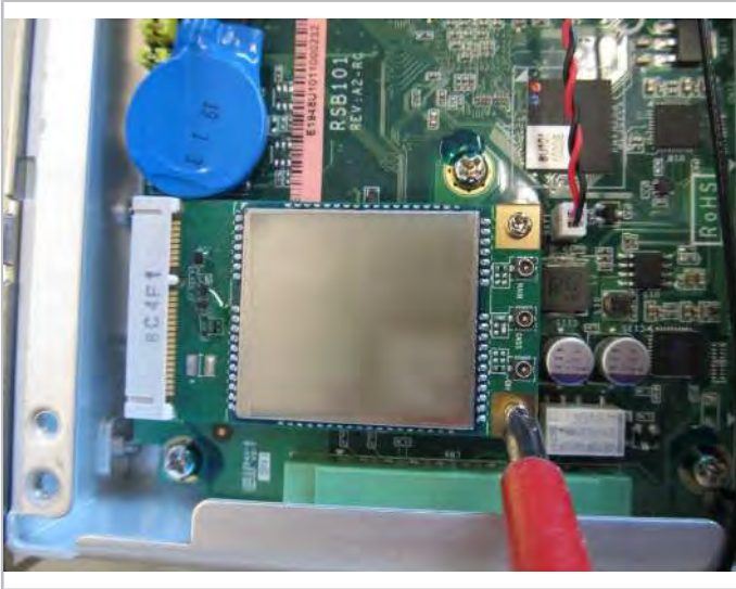
Fig. 16: Open the screws on the GSM module.
