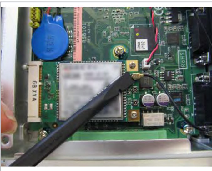
Fig. 15: Remove the antenna cable from the GSM module.
